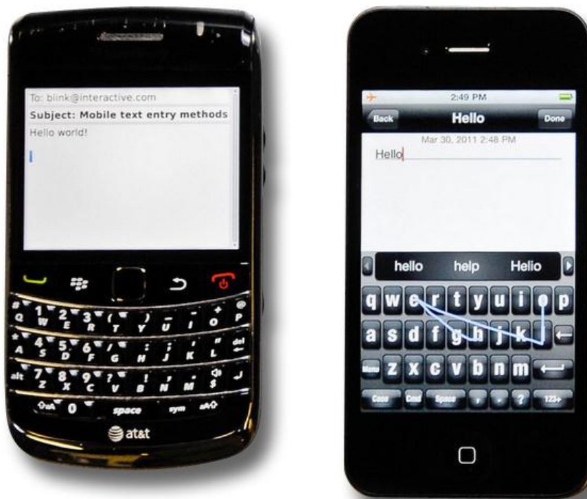
Figure 1. The BlackBerry Bold physical keyboard (left) and the ShapeWriter touchscreen keyboard (right).
